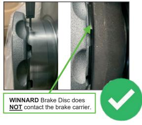
Attention to design and machining detail are vital to ensure the correct fit and operation.
